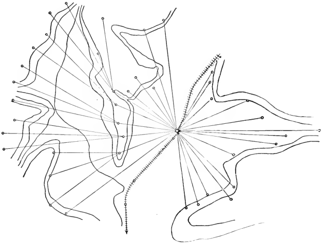
FIG. 68. — A Logging Chance showing the Use of an Overhead Cableway System in bringing Timber over a Ridge by relaying
